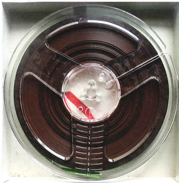
Figure 8.02 The magnetised data dots are stored in series along the length of the magnetic tape
