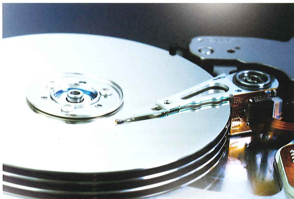
Figure 8.03 In a hard disk, an arm moves back and forth across platters to access data in different tracks
