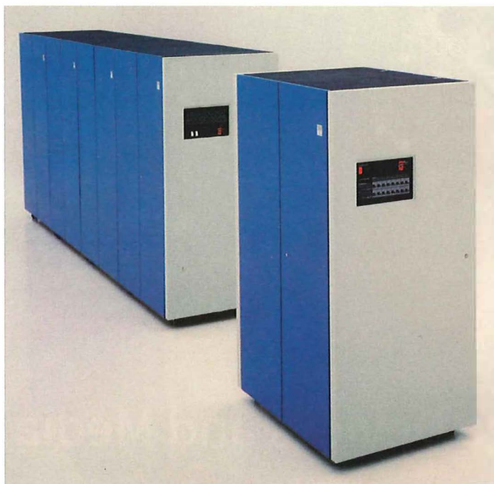
Figure 8.01 The IBM 3380 was the first storage device to have a capacity of 1 gigabyte
